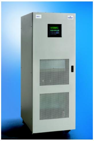
The Liebert FS is configured as a two-terminal plus ground DC flywheel power system and is used as a functional replacement for or an availability supplement to a bank of chemical batteries for an Uninterruptible Power System. Like a chemical battery bank, Liebert FS receives charge and float power from the two terminal UPS DC bus and returns power to the same DC bus whenever the bus voltage droops below a programmable threshold level.
